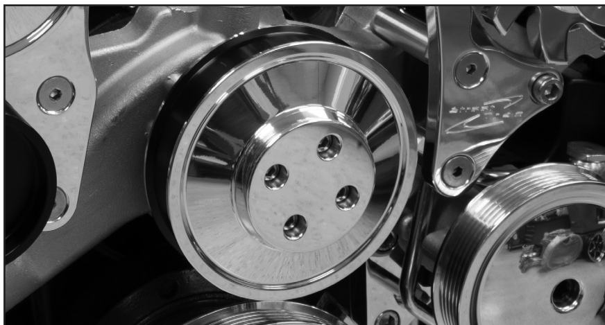
Figure 12: Install Water Pump Pulley
